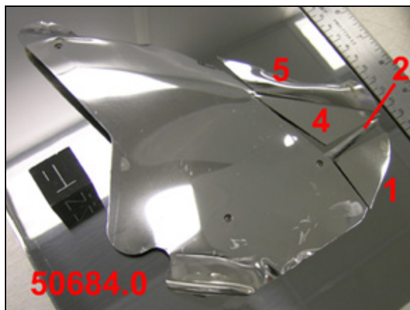
Fig. 1. Polished aluminum collector after subdivision in 2005. Portions 1, 2, 4, and 5 were previously imaged. Imaging of portion 50684.0 is in progress.
